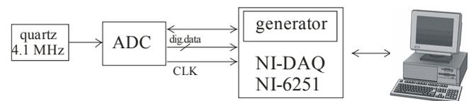
Fig. 4. ADC test set-up
