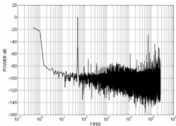
Fig. 6. a) Power spectrum of input signal; Hanning window
