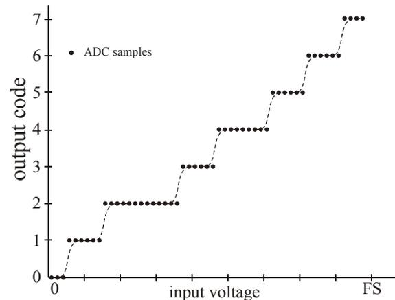
Fig. 2. ADC samples from linear ramp histogram test
