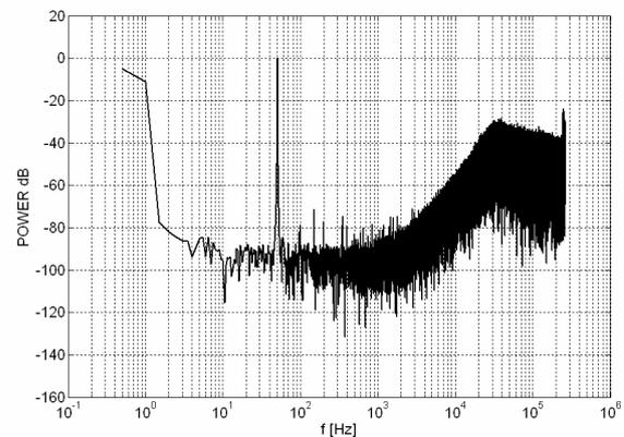
Fig. 6. c) spectrum of the ADC output signal behavioral level; Hanning window
