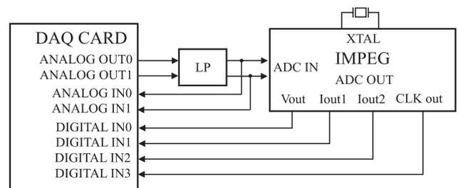
Fig. 5. Block diagram of interconnection between acquisition card and IMPEG
