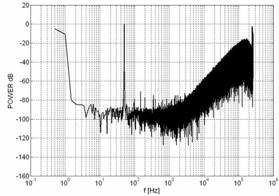
Fig 6. b) spectrum of the ADC output signal; Hanning window
